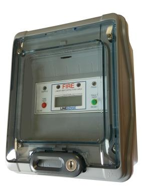
The Digital Location Interface (DLI) monitors the Linear Heat Detection (LHD) cable and when activated identifies the location of the alarm. The distance in meters is then displayed on the 3½ digit LCD. Providing detection and location along the complete length of the LHD cable.
